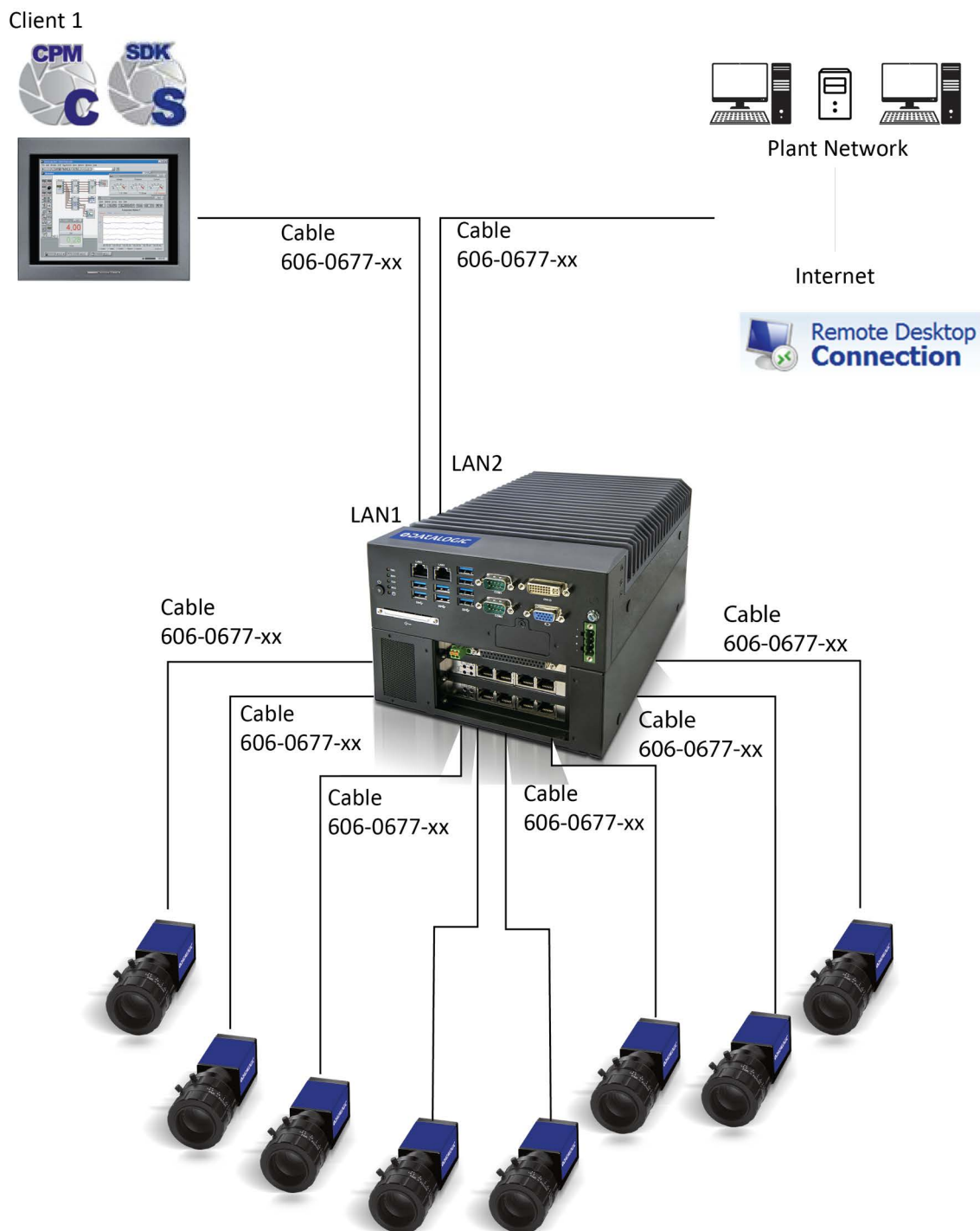
Figure 3 External LAN Connections using LAN1 and LAN2 (Basic configuration)
